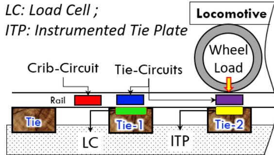
Figure 1: Instrumentation Layout
